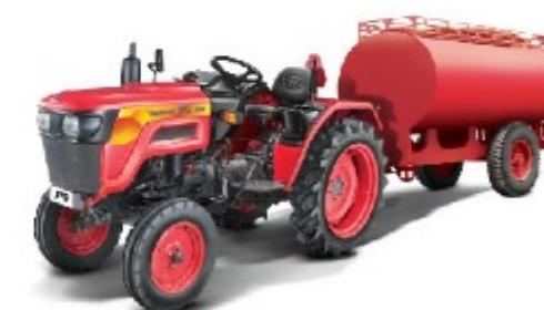
Water Tanker: Pulling power of 3 tonnes
